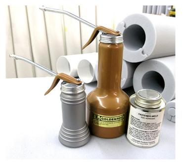
All seams for 300 & 800 Series jackets, both straight lap joints and circumferential lap joints, should be glued with Fastener Weld. This is important in both indoor and outdoor applications to prevent the ingress of water or wash down fluids into the TechLite<sup>®</sup> foam. In below ambient piping applications and severe wash down environments, all seams should be over-sealed with a factory approved RTV sealant to guarantee a positive vapor barrier seal.
