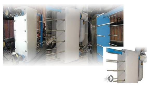
Adaptable insulation packages for plate and frame heat exchangers allowing on-site installation. Provides personnel burn protection, condensation control, and reduces heat loss. Closed cell foam is used in below ambient applications whereas high temperature open cell melamine foam is used for above ambient applications. Most units feature removable panels via Velcro® closures to simplify maintenance.
